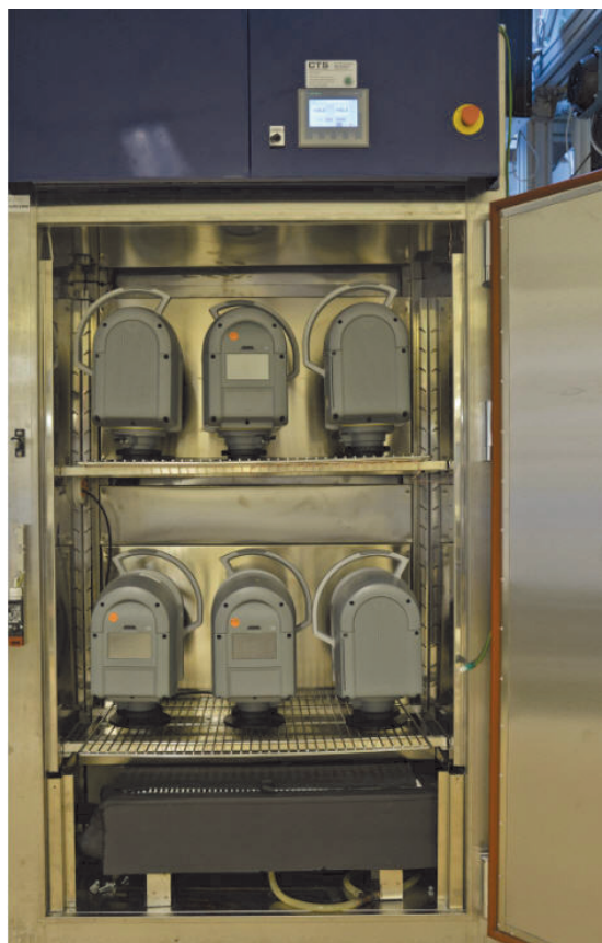
Figure 12: Thermal chamber to induce environmental stress with extreme temperatures
