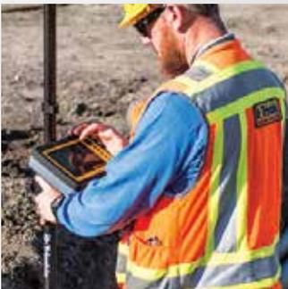
**Trimble® Field Link** features task-based workflows, customizable views and a touch screen user interface designed to optimize the information presented, and extends field layout capabilities. In addition to the advancements made in performing layout specific tasks, it adds reporting routines to record and track layout productivity as well as the ability to document existing site conditions.
