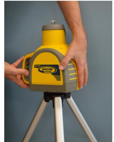
To remove laser from tripod for storage, it is easier to turn the laser while attached to tripod base
