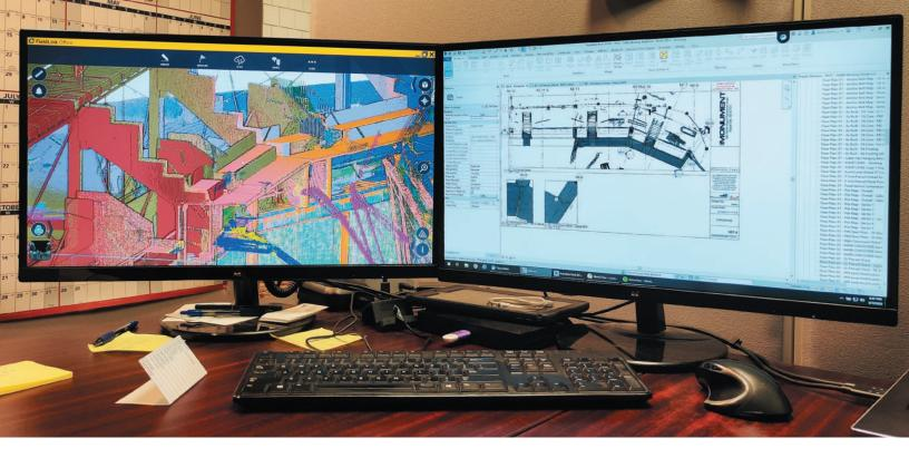
By streamlining their workflow with the X7, Mortenson/Scull can efficiently scan every slab on metal deck (SLOM) and slab on grade (SOG) before placing concrete, ensuring with 99% certainty that the embedded components are in the planned location.
